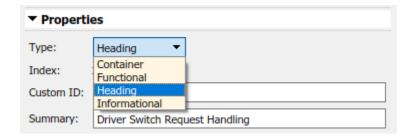
To select the custom link type, navigate to the **Links** view and select a link. Select the custom link type from the **Type** drop-down list in the **Properties** pane.
