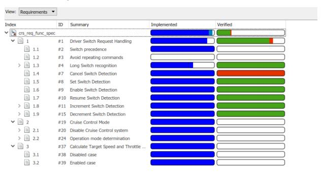
There are two workflows for justifying requirements in Simulink Requirements. You can either create a new justification object and link requirements to it or use an existing justification object and link requirements to it.
